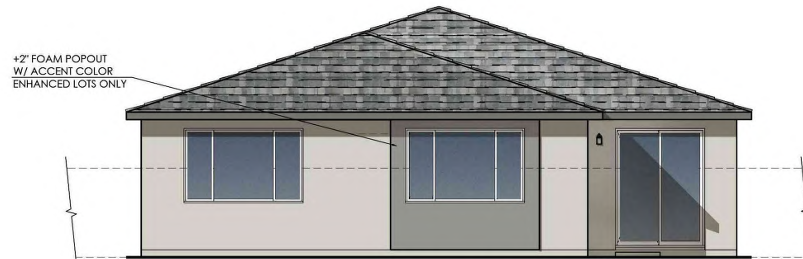
Rear Elevation "Enhanced"
